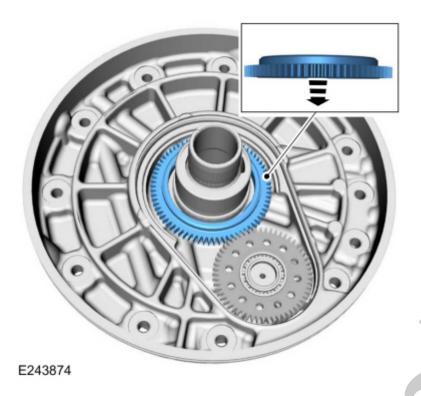
270. Install the front support cover by pressing down evenly by hand.
