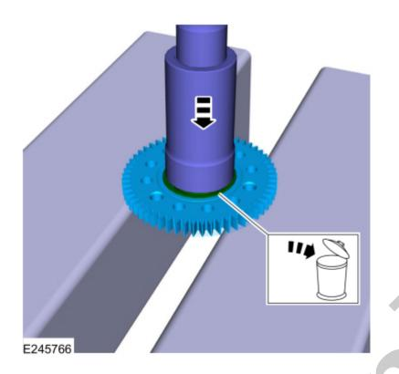
264. Remove and discard the stator support seal.
