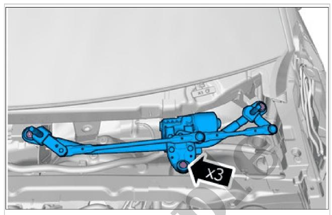
**Torque:** M6, 10Nm Remove the screws. Remove the marked part.
