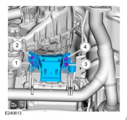
11. Install the LH (left-hand) isolator cap and the bolt.
