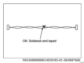
• Never bypass the repair point with wire. (If it is bypassed, the turnout point cannot be separated and the twisted wire characteristics are lost.)
