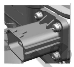
10. CX482/CX483 - PHEV - High Voltage Battery Cable to Secondary On-Board Diagnostic Control Module A (SOBDM) (6-way)
