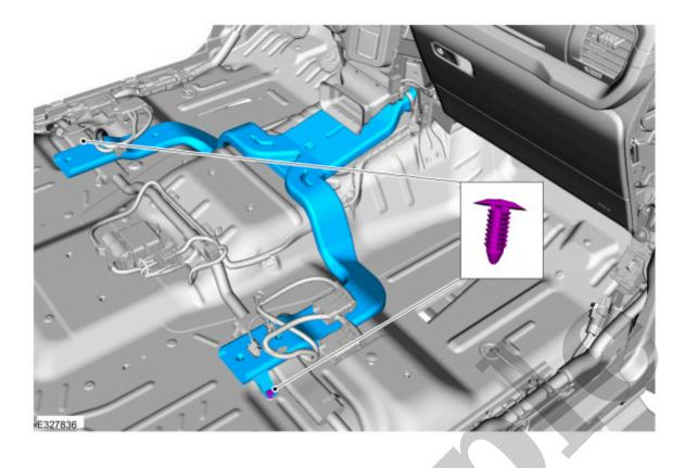
20. Disconnect the electrical connectors, release the harness retainers and postion aside the harness.
