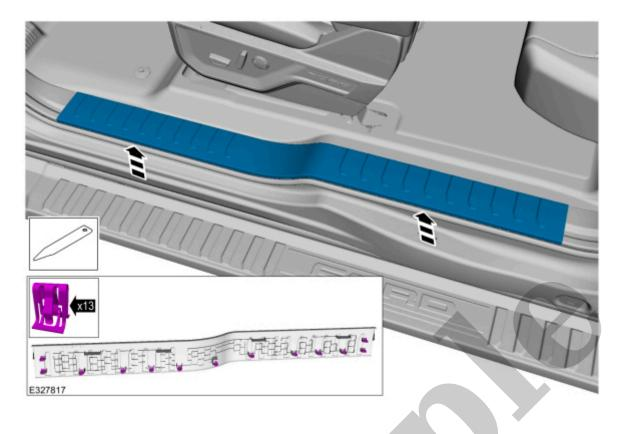
9. Release the clips and remove the LH (left-hand) lower cowl trim panel.
