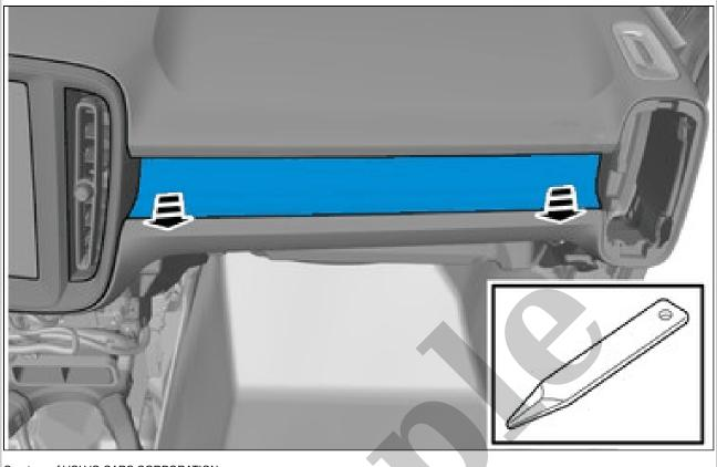
Use: Interior trim remover Remove the part carefully Remove the marked part. VEHICLES WITH DECOR ILLUMINATION
