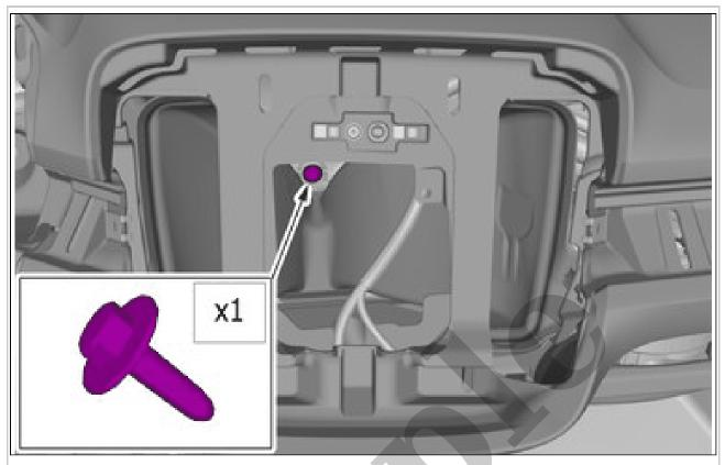
Remove the screw. **Torque:** Dashboard, to crossmember, 3.5Nm
