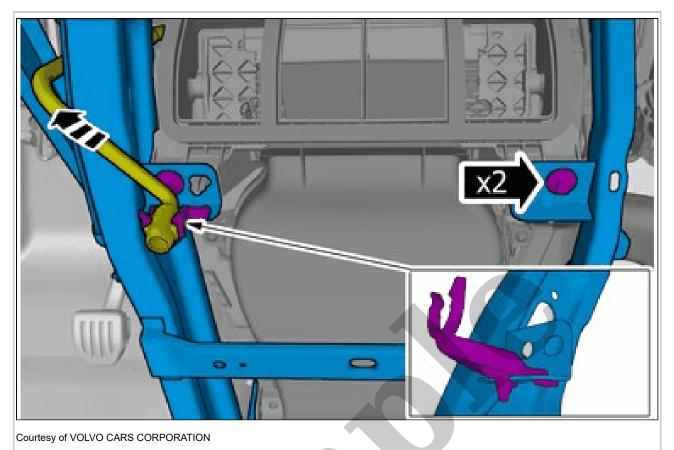
Remove the screws. **Torque:** Cross member, to Climate unit, 5.4Nm Remove the marked part.
