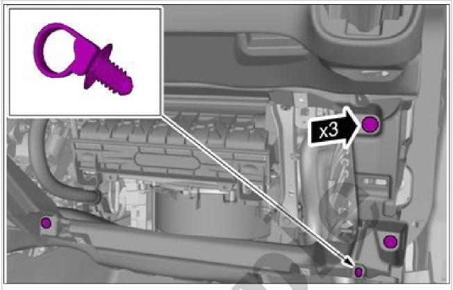
Remove the screws. **Torque:** Dashboard, to crossmember, 3.5Nm Remove the cable harness clips.
