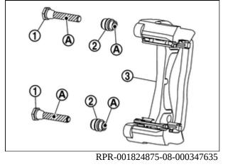
7 Install cylinder body to torque member and tighten sliding pin bolts to the specified torque.
