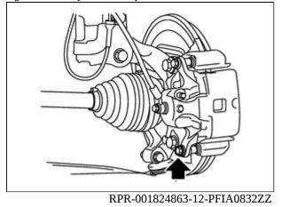
7 Check front disc brake for dragging, while depressing brake pedal several times. Refer to <u>Inspection and Adjustment</u>.
