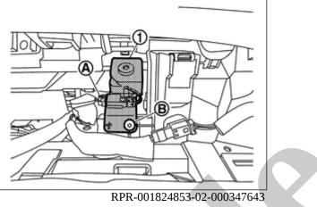
3 Remove mounting screw B and the remove warning buzzer 1.
