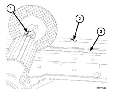
13. Cut off the flange (3) with a cut-off wheel (1) or equivalent.
