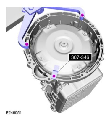
4. Using the special tool, remove the torque converter.
