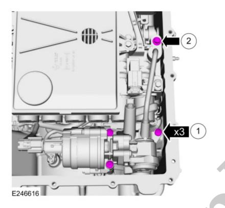
25. Connect the transmission fluid auxiliary pump electrical connector.
