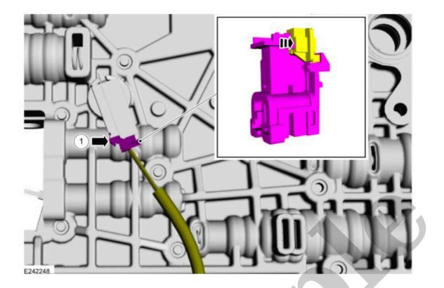
3. Install the main control valve body.
