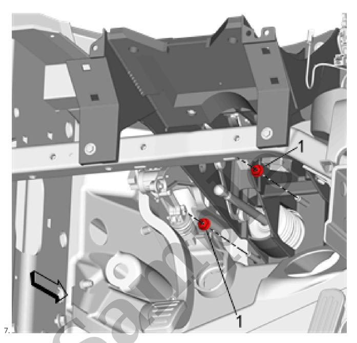
Remove the power brake booster nut (1).
