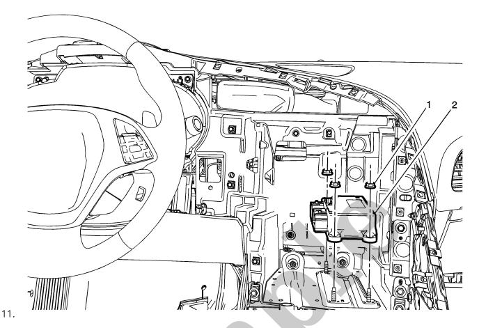
Restraints Control Module(2) »Install— Restraints Control Module Replacement
