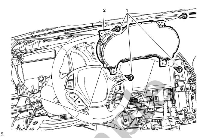
Remove the instrument cluster (2). Instrument Cluster Replacement
