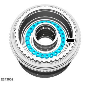
146. Lubricate the new D clutch balance dam seals with petroleum jelly.
