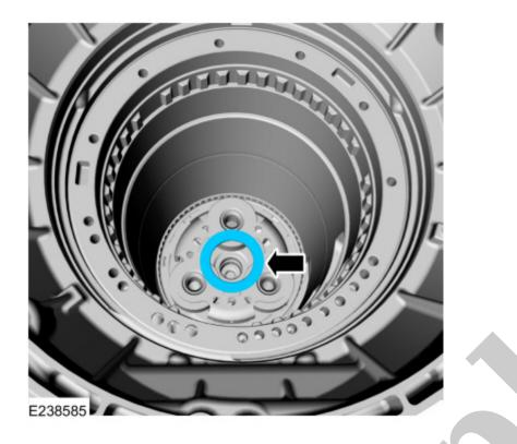
27. Remove the A clutch assembly. If the clutch plates are not excessively worn or damaged, they can be reused.
