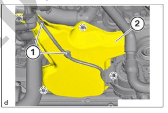
(a) Thread in and position the cylinder block cover (2).
