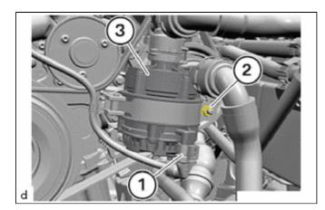
(b) Tighten the nut (2) on the holder.
