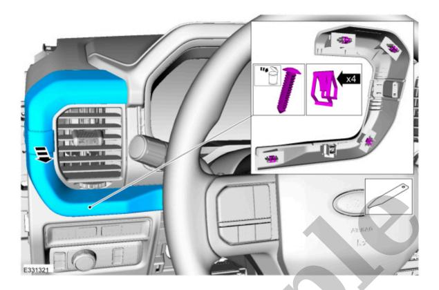
4. Release the clips and remove the lower steering column closeout panel.
