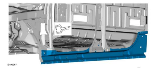
5. Drill 6.5 mm holes for fasteners.
