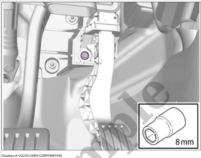
Remove the screw. The part is to be reused.
