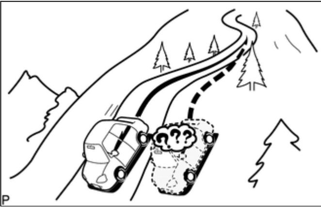
(6) When the vehicle makes a continuous turn (e.g. 360, 720, 1080 degrees), the current vehicle position mark may deviate from the correct position.
