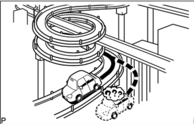
(7) When the vehicle moves erratically, such as constant lane changes, the current vehicle position mark may deviate from the correct position.
