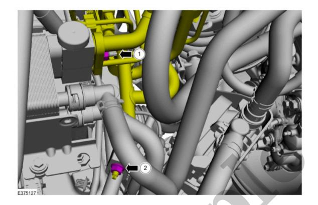
5. 1. Remove the A/C (air conditioning) refrigerant line nut and disconnect the fitting.
