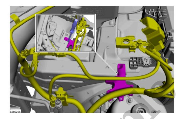
7. 1. Remove the thermostatic expansion valve manifold tube assembly bracket retainer.
