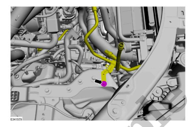
11. Remove the thermostatic expansion valve manifold tube assembly bracket retainer.
