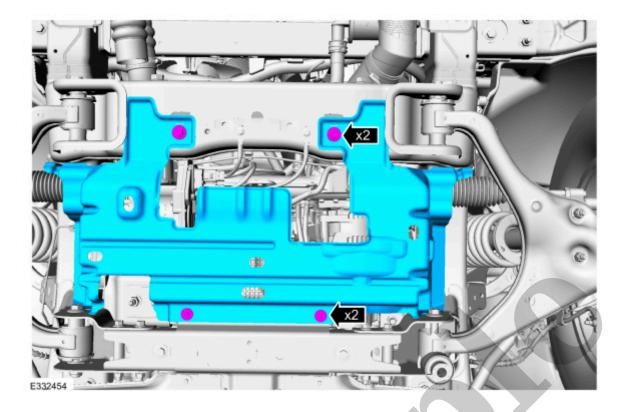
14. Remove the bolt and the pin-type retainer.
