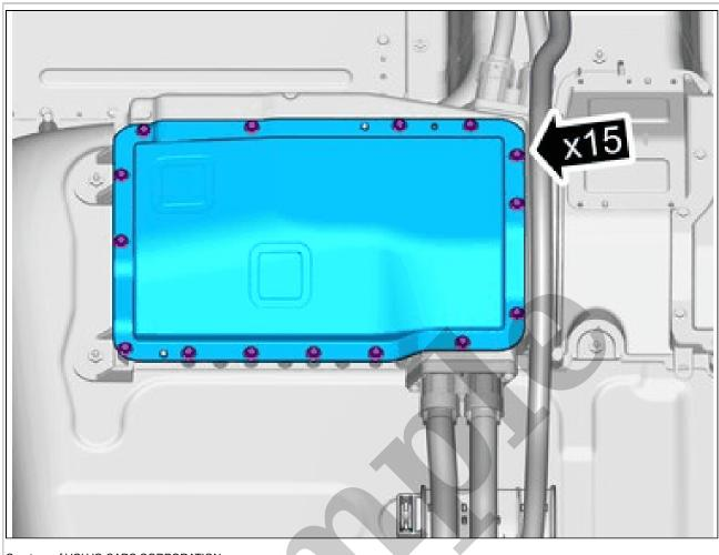
Remove the screws. Remove the marked part.
