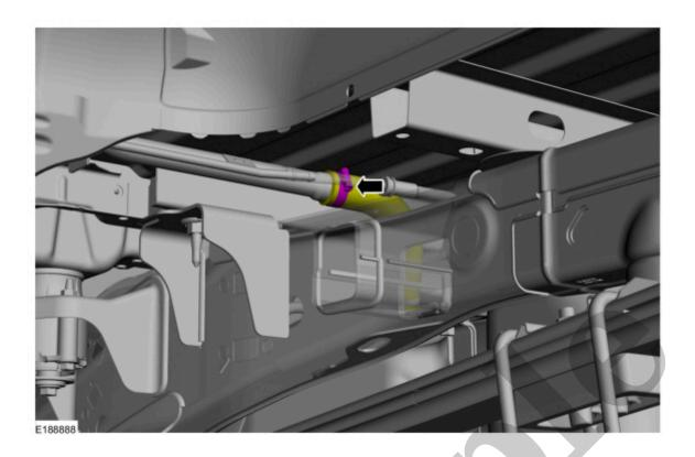
4. Disconnect the fuel tank filler pipe vapor tube quick release coupling.
