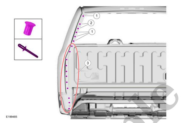
30. Metal finish all sectioning seams using typical aluminum metal finishing techniques and a fiber-based filler.
