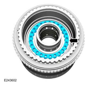
119. Remove the D clutch piston. Use compressed air into one oil passage hole while plugging the hole on the opposite side.
