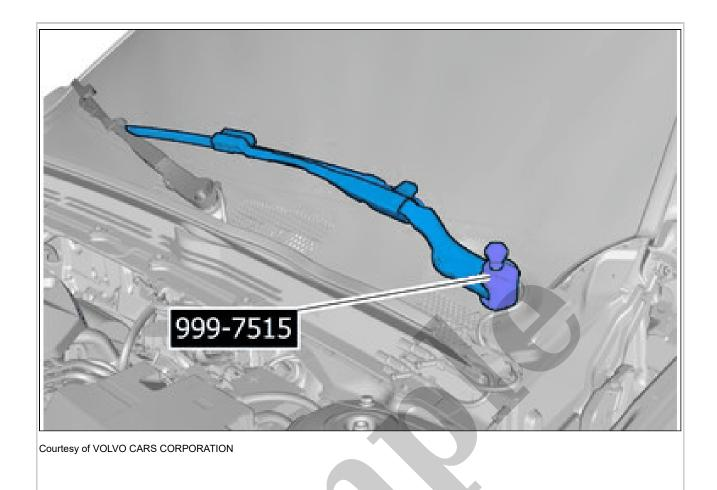
Special Tool: 999 7515 Puller Remove the marked part. On both sides.
