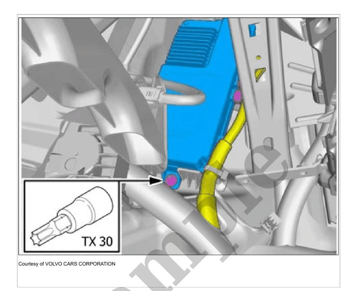
Remove the screw. Remove the marked part.
