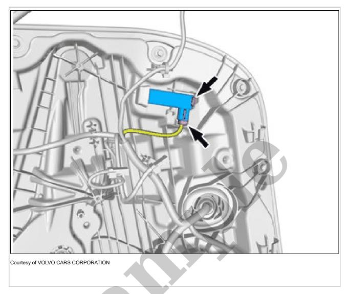
Remove the marked part. Disconnect the connector.
