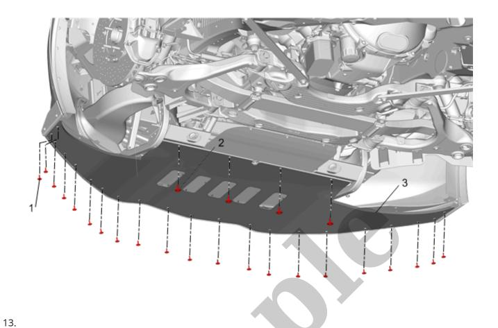
{ If equipped }Front Bumper Fascia Air Deflector(1) »Install— Front Bumper Fascia Air Deflector Replacement
