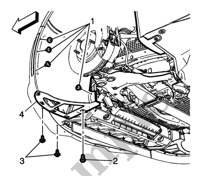
Install the front wheel house bolts (1, 2, 3). Front Wheelhouse Liner Replacement
