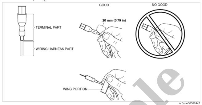
5.Insert the tool into the female terminal, then slowly pull it out.
