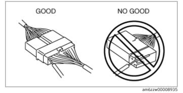
• Inspect the terminals of waterproof connectors from the connector side since they cannot be accessed from the wiring harness side.
