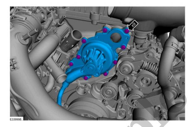
14. Remove and discard the coolant pump gasket and O-ring seal.
